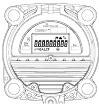
Segment Test View
