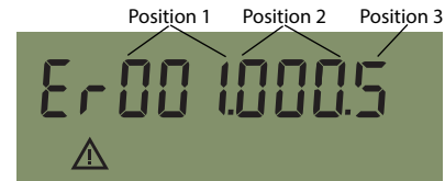
Figure 12: Alarm and operating mode screen in storage mode
