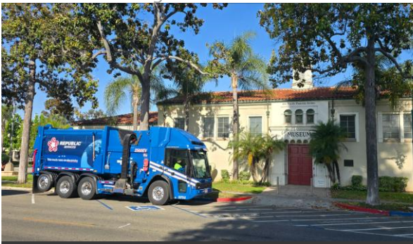
Figure 6. EV Automated Side Load Collection. Provides a quieter, cleaner and safer hauling vehicle.
