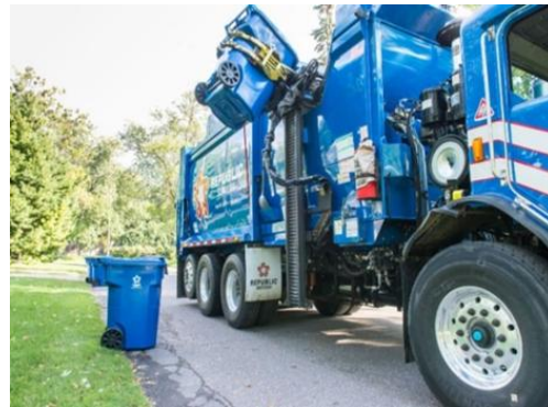
Figure 13. Automated Side Load Collection. Provides a cleaner, safer, more efficient residential collection.
